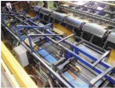
• SA Pine Edger Infeed with Joescan sensors
