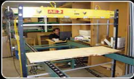
Above : A&E Workshop Test bench with LMI Chromoscan 3350 Sensors and some image capture results
