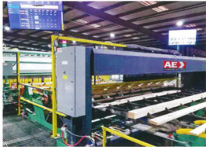
● A high density scanner in operation in the United States.
